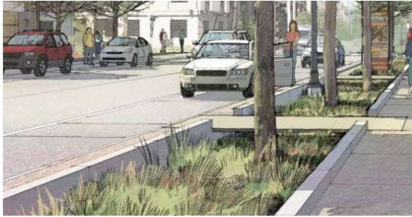
Flow through planters create opportunities for habitat and ecology to be created and provide the public with shade
